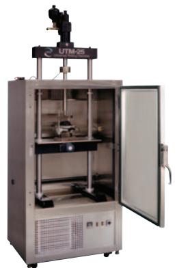
UTM-25 with Environmental Chamber
